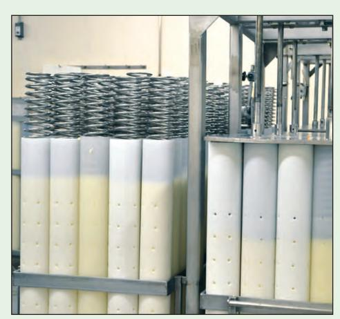
How do they make round deli loaves of cheese? Curds are inserted into round cylindrical molds – and then pressed using spring-type mechanisms pushed down from above by a stainless-steel mechanism. Round deli loves may be produced in 4-inch and 6-widths. After pressing the curds into 39-inch lengths, the tube-shaped deli loaves are cut into 12-inch or 18-inch lengths, depending on end-users specifications.
